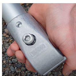
3. Put on the second half and fasten hex bolt
